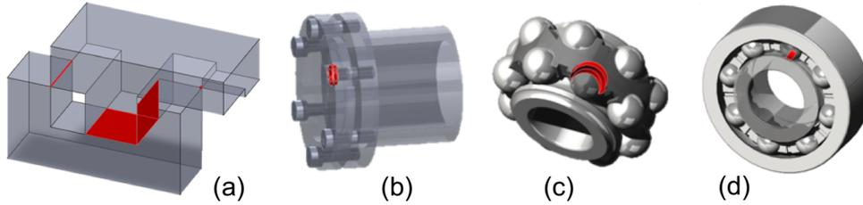
**Fig. 2. Possible contacts between parts of a CAD assembly model: (a) contacts of type Surface, Curve and Point, (b) Unsolved contact type, (c) volumetric interference solved as Surface contact type, (d) volumetric interference solved as Curve contact type.**
