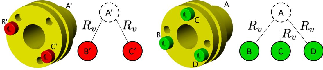
Fig. 4. Example of two assembly models with a different number of screws, and their EAM attributed multi-graphs  $G_1$  and  $G_2$ .
