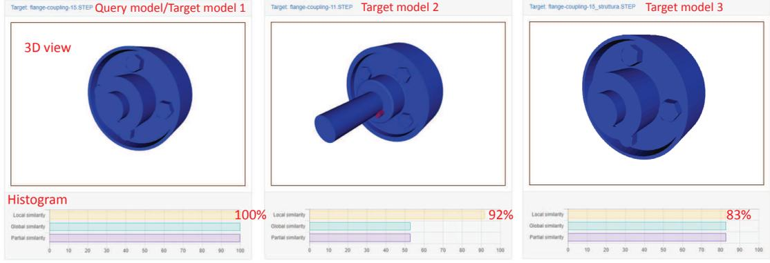
Fig. 8. Example of two target models (middle, right) retrieved from a given query model (left).
