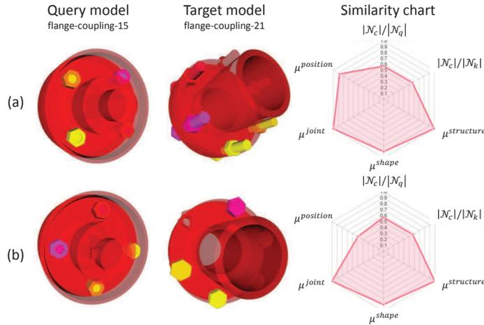
**Fig. 9.** Two different cliques (a, b) when comparing the target model (#4) to the query model (#1) in Table 2. The arrangement of the parts is different which is reflected by different values of  $\mu^{position}$  in the radar charts.
