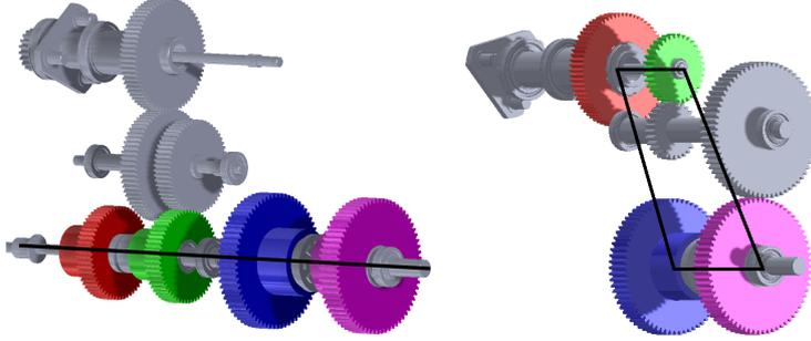
Fig. 7. Example of assembly models with similar parts arranged according to different configurations.
