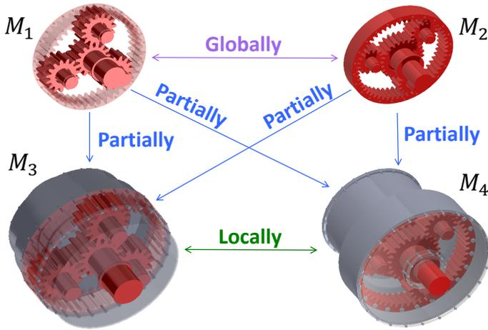
Fig. 1. Example of different similarity levels for the retrieval of CAD assembly models (local, partial and global).
