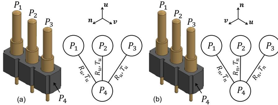
Fig. 6. Two instances of the same object embedded in two different reference frames: (a) query model, (b) target model.
